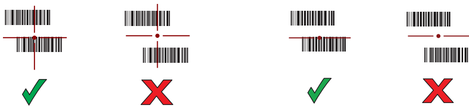
Figure 87 Pick List Mode with Multiple Barcodes in Aiming Pattern: Standard and Extended Range
